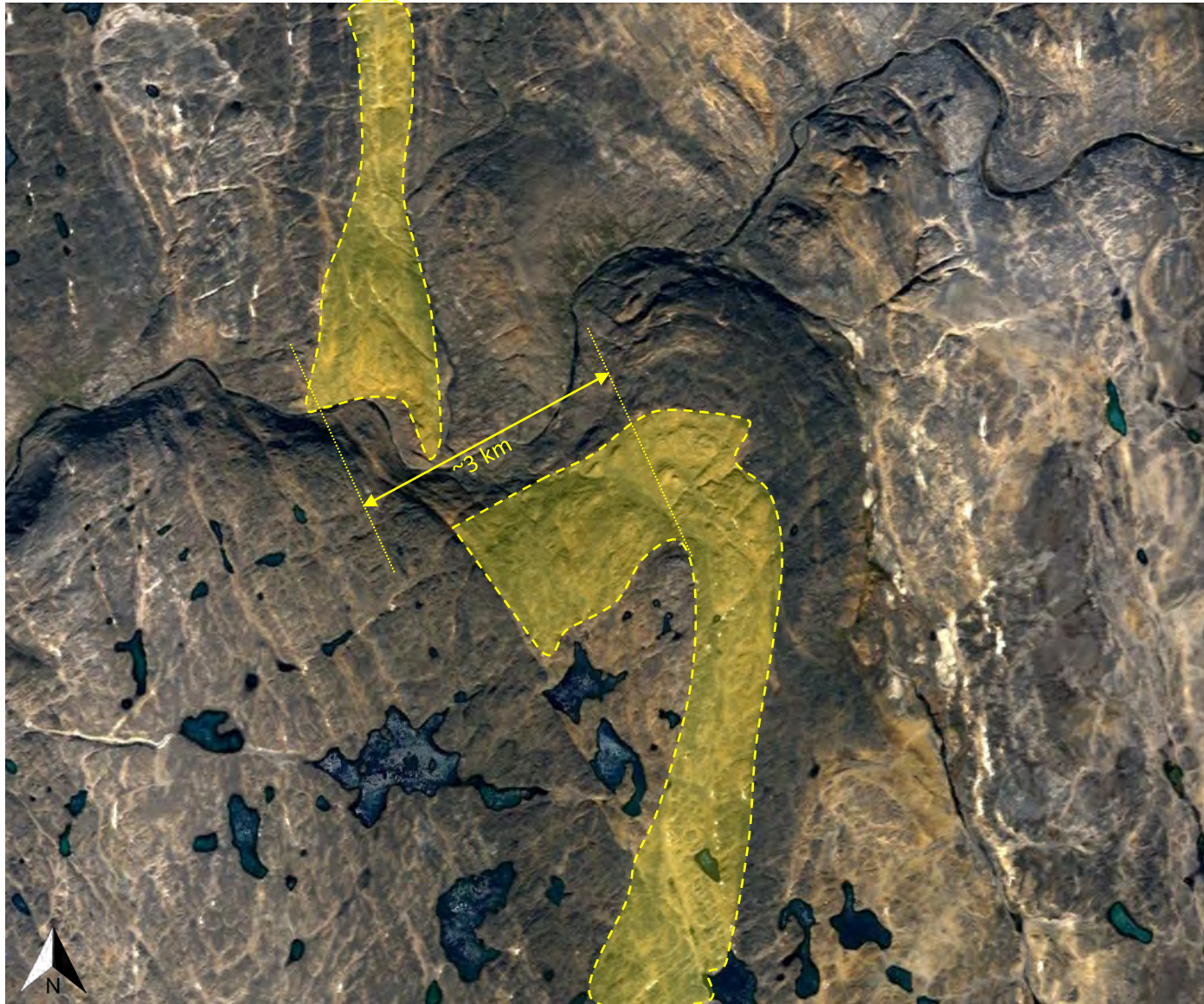
Possible contortion of a marker band showing about 3km of offset to potential fault movement
